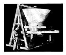
The entire bin and discharge table revolve. As the cylinder and plate rotate, the plow continuously removes a stream of material from the bottom of the mass of the cylinder, discharging it off the top of the plate. Discharge rate can be varied by altering the thickness of the plow and the speed at which the feeder turns.
