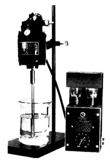
is constant over the entire speed range. An increase in power requirement is automatically signaled to the control unit, which supplies D.C. power in stepless variation to the motor.
